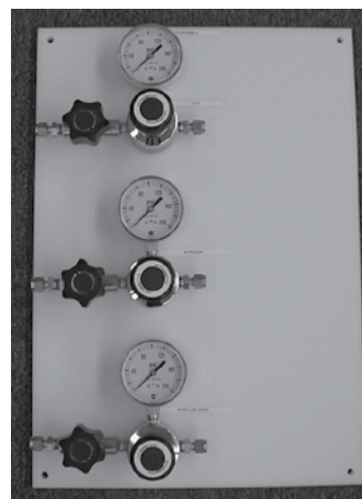
three-regulator vertical panel configuration
