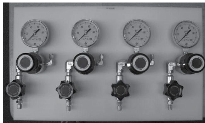
four-regulator horizontal panel configuration
